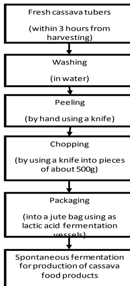
**Figure 1.** Scheme of cassava pieces natural lactic acid fermentation processing
