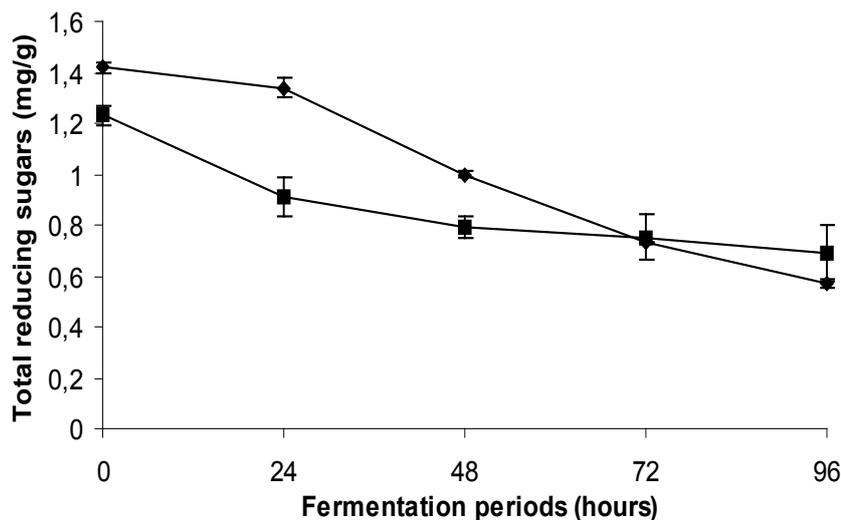
**Figure 4.** Change in total reducing sugars during cassava lactic acid fermentation. Symbols:  $\blacklozenge$ , sweet variety roots,  $\blacksquare$ , bitter variety roots. Error bars represent standard deviation
